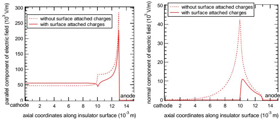
**Figure 2.** Electric field along the insulator surface
