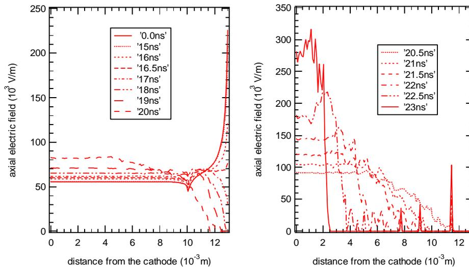
**Figure 4.** Electric field distribution along the axis
