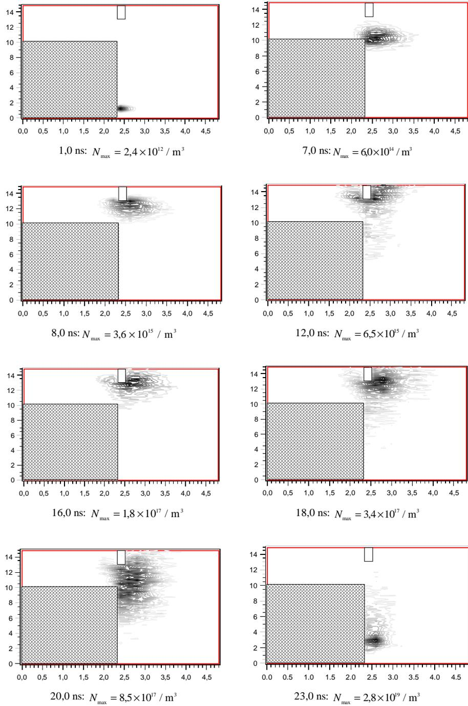
**Figure 3.** Electron avalanche and streamer development
