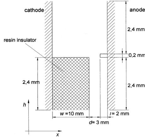
Figure 1. Needle-plane configuration inserted by a resin insulator with cut plane
