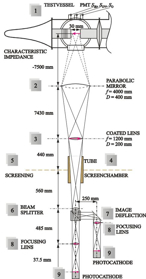
Figure 1: Electro-optical test set up and test vessel.
