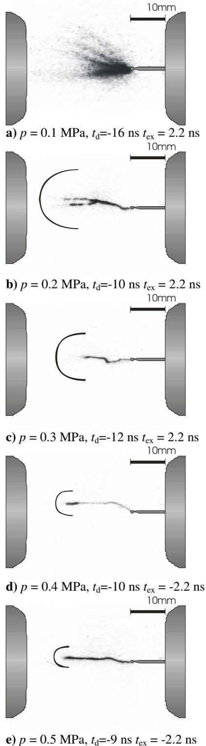
**Figure 2:** Pressure dependent prebreakdown development for 20/80 %  $\text{N}_2\text{O}/\text{N}_2$  gas mixtures  $f_{\text{VFTO}} = 1 \text{ MHz}$ , gap width  $d = 30 \text{ mm}$
