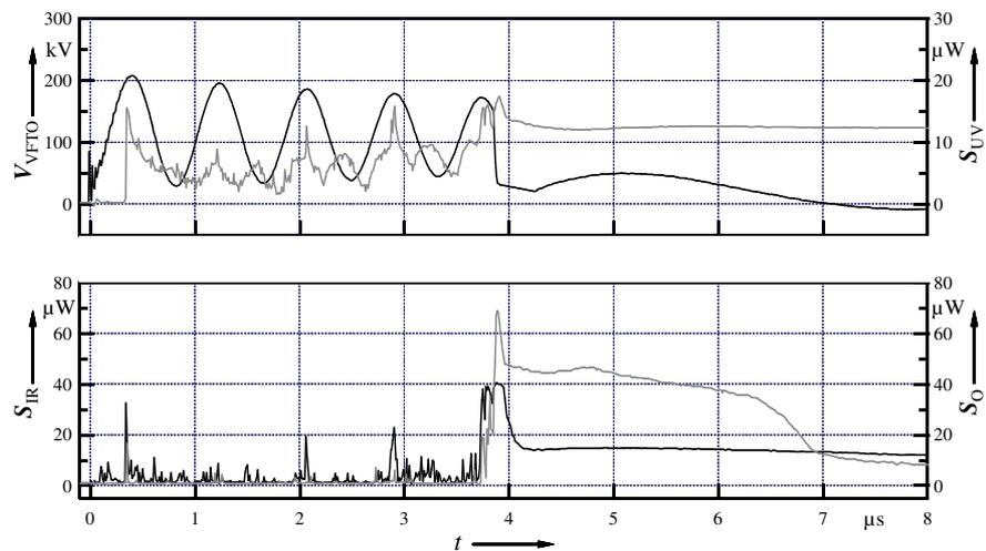
**Figure 4:** Typical electro-optical prebreakdown development signals ( $S_{UV}$ ,  $S_{IR}$  and  $S_O$ ) for 20/80 %  $N_2O/N_2$  gas mixtures,  $p = 0.3 - 0.5$  MPa,  $f_{VFTO} = 1$  MHz. A combined precursor and high frequency mechanism was often observed, as shown in this figure at a pressure of  $p = 0.5$  MPa.
