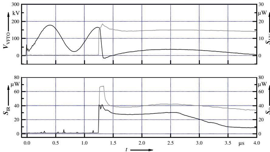
**Figure 3:** Typical electro-optical prebreakdown development signals ( $S_{UV}$ ,  $S_{IR}$  and  $S_O$ ) for  $p = 0.1 - 0.2$  MPa, 20/80 %  $N_2O/N_2$  gas mixtures,  $f_{VFTO} = 1$  MHz.
